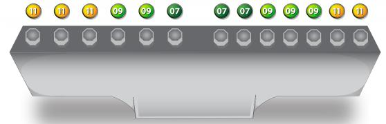
8" Medium Aggressive Set Up 5.41GPM @ 36K /5.74 GPM @ 40K PSI
